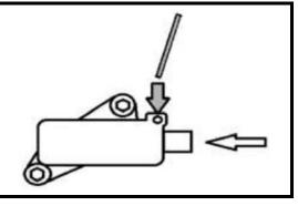
Crankshaft Timing Pin, to be used as OEM VM10339
