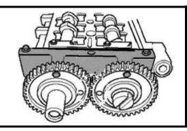
Camshaft Locking Tool (2) for left cylinder head, to be used as OEM VM10338-2
